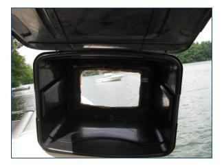
The scope has a large view area, approximately 10" x 15". The Plexiglas is glued to the inside of the tub with liberal amount of glue, weighted and left to dry overnight.
