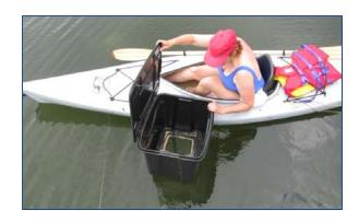
The tub scope can be towed behind your kayak or canoe then pulled alongside for viewing. The hinged top can be manually adjusted to shield the Plexiglas view window from the sunlight.
